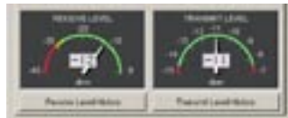
Realtime measurement of the receive and transmit levels of the optical transceivers
